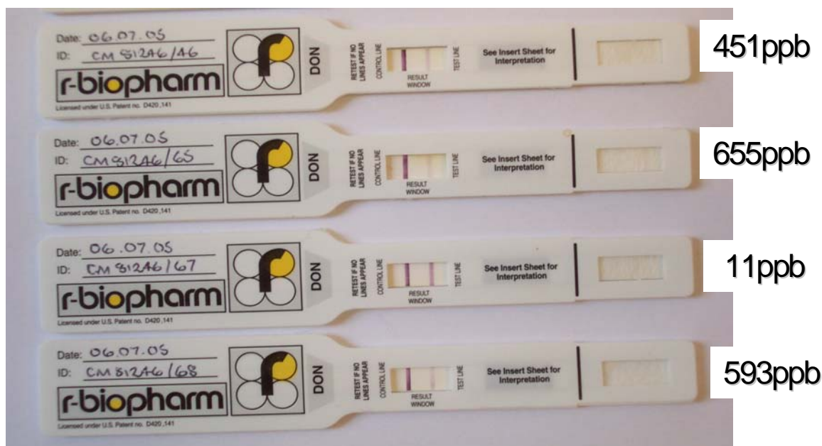
Figure 1: Results of Quick DON test carried out on wheat extracts with low DON levels ( reference values quoted in ppb)
